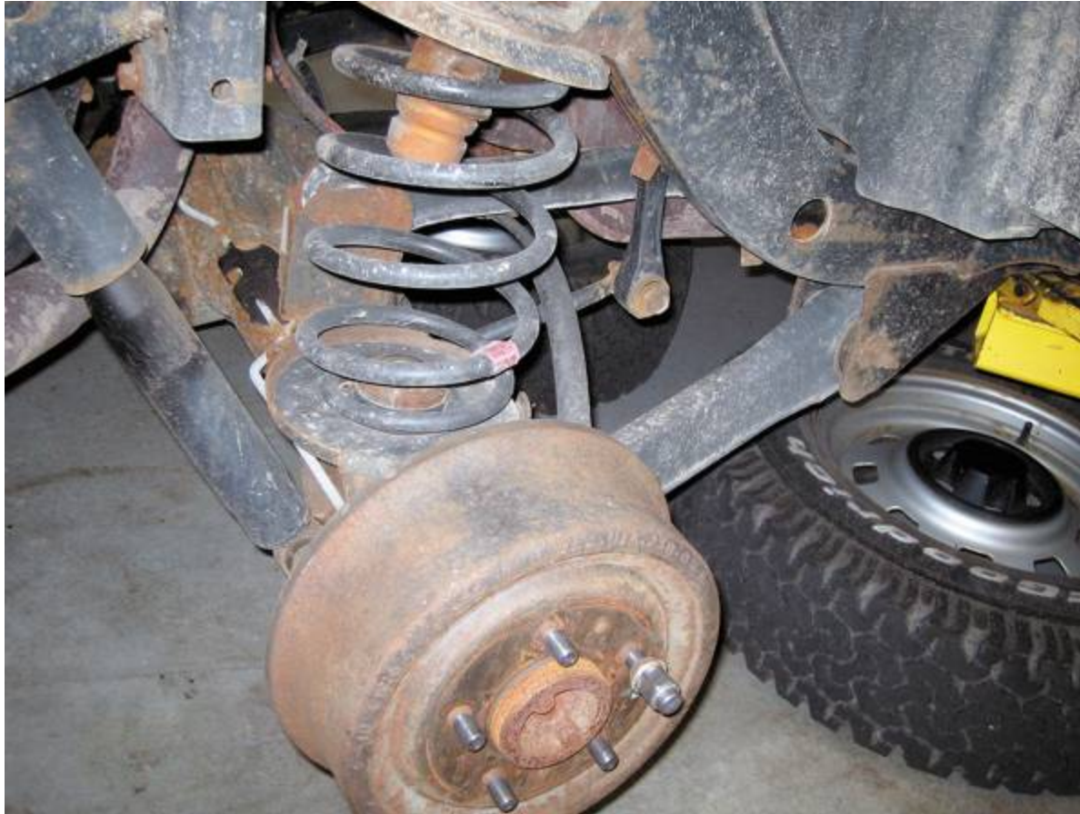
FIGURE 26–20 The shock absorber needs to be disconnected before removing the coil spring. Installation is the reverse of removal procedure.
