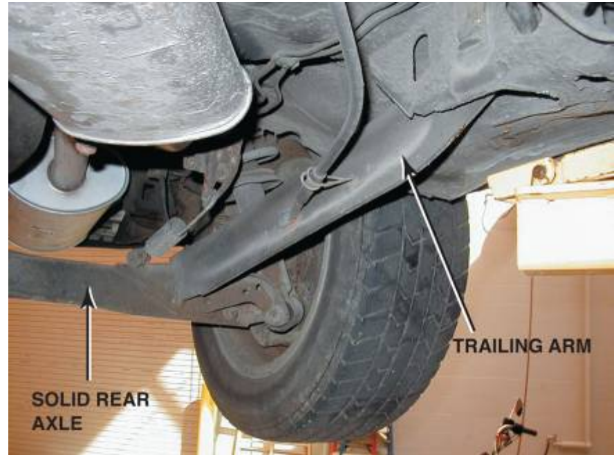
FIGURE 26–6 A trailing arm rear suspension with a solid axle used on a front-wheel-drive vehicle.
