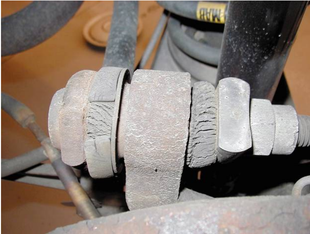
FIGURE 26–17 Check all rubber bushings for excessive cracking.
